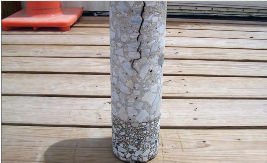
Figure 2. Deep Plastic Shrinkage Crack (below mid-depth).
