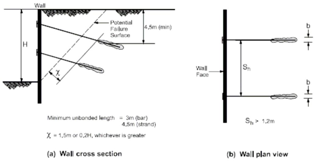
**Figure 2. Minimum Distance Between the Failure Surface and the Start of the Grouted Section.**
