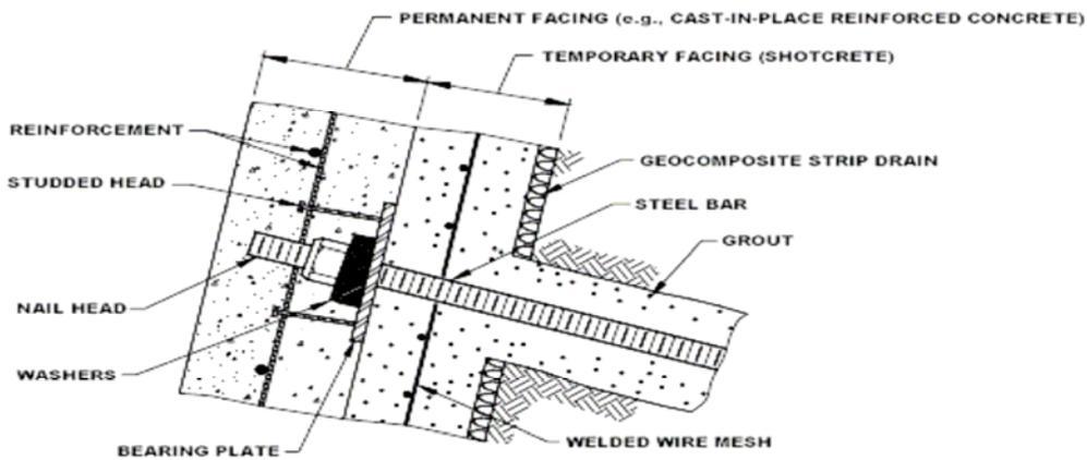
Figure 3. *Typical cross section of a soil-nail wall.*
