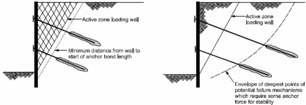
**Figure 1. Cross sectional view of the probable tiebacks.**
