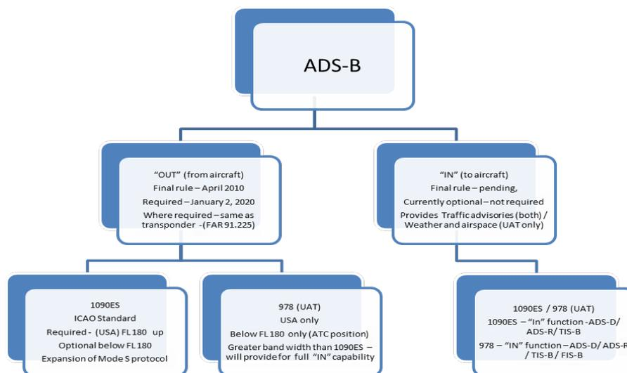
Note that the OUT function is required by FAR 91.225 on 1/2/2020. This means as a minimum you must be capable of transmitting a position derived from a WAAS enabled IFR certified GPS to ATC using either protocol. The 1090ES protocol is required in class A airspace or outside of the USA at any altitude. The IN function is not required by FAR, however IN will provide traffic near your aircraft by three methods:
