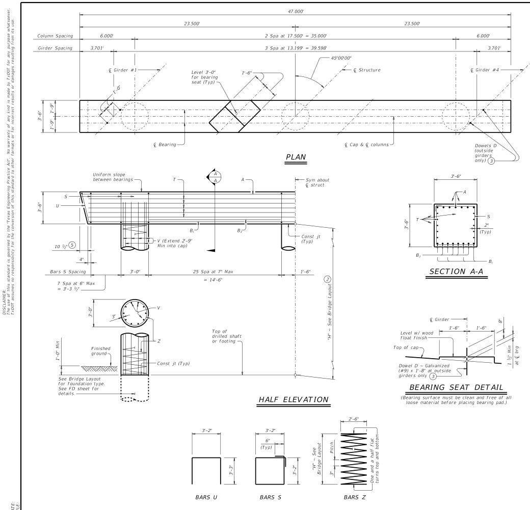
1) Quantities shown are based on an "H" value of 36'. For each linear foot variation in "H" value, make the following adjustments: Bars V length, 1'-0" Bars Z length, 31'-5"
