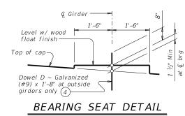
(Bearing surface must be clean and free of all loose material before placing bearing pad.)
