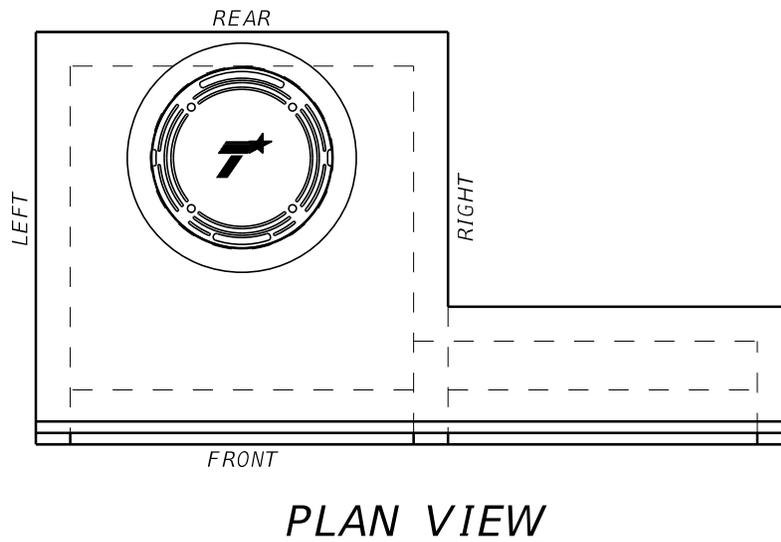
Figure 2: Extension Placement on PCO Inlet
