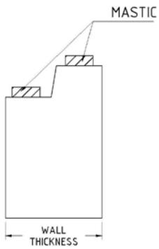
Figure 6: Standard Precast Joint Detail
