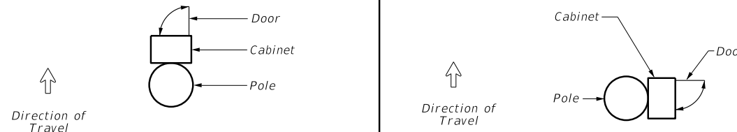
Orientation of Type 2 Cabinet on ITS Pole (Typical)
