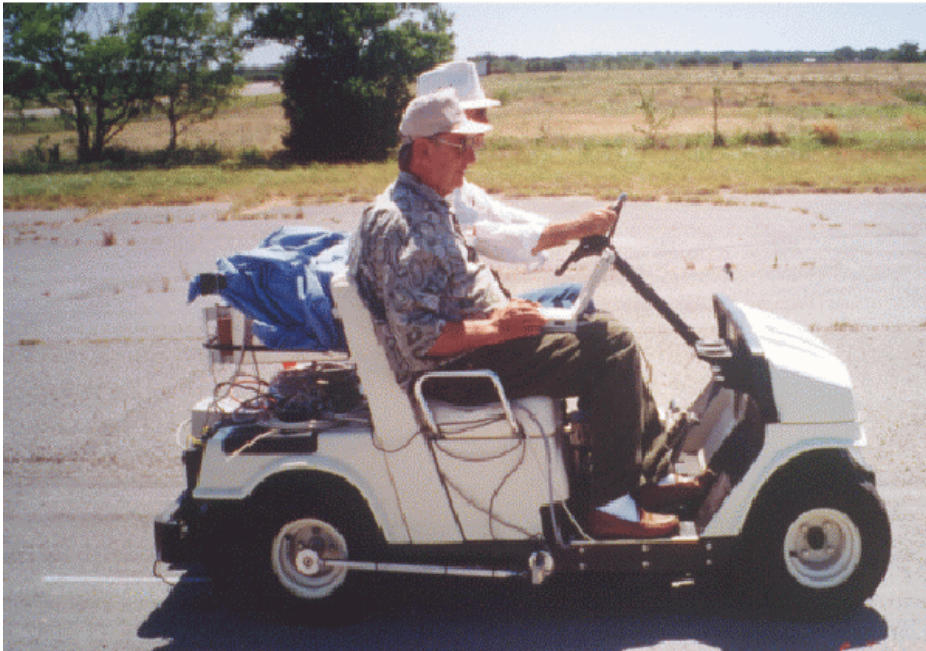
Figure Error! No text of specified style in document. -2. Illustration of a lightweight inertial profiler developed by TxDOT.
