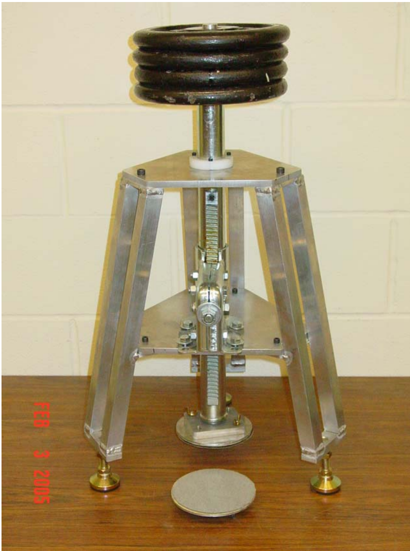
Figure Error! No text of specified style in document. -1. Tack Coat Pull-off Device.
