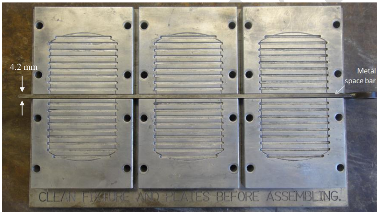
Figure 5 —Mounting Jig, Base Plates, and Spacer Bar
