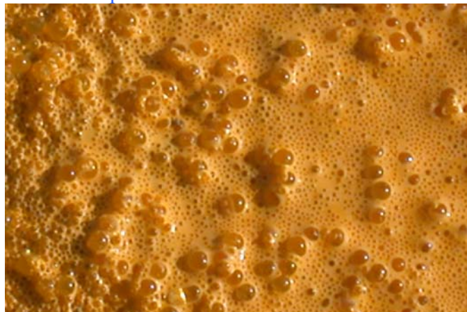
Figure 5. Epoxy application with Type IV and Type I beads
