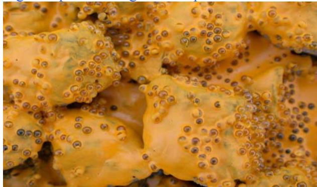
Figure 1. Picture of Type III beads in traffic paint on a Grade 3 seal coat
