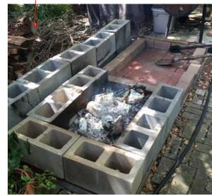
Figure 5. Carbonizing samples.
