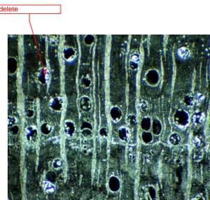
Figure 7. Transverse plane of mesquite wood charcoal (45x).
