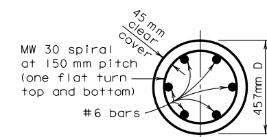
ANCHOR DETAIL - SECTION E-E
