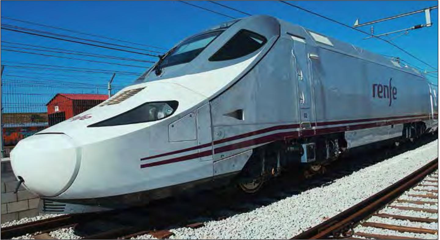
The RENFE Class 130, a high speed dual gauge, dual voltage trainset consisting of eleven Talgo VII tilting coaches and two power cars.
