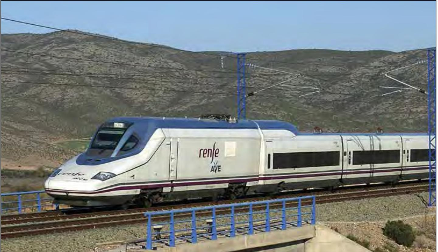
**Talgo 350 Train.** This series of trains are designed to reach a speed of 350 km/h (220 mph), although present lines and commercial services limit the speed at 330 km/h (205 mph).
