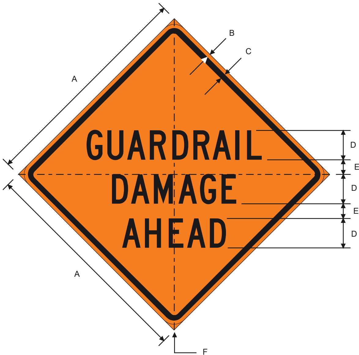
CW21-17T GUARDRAIL DAMAGE AHEAD
