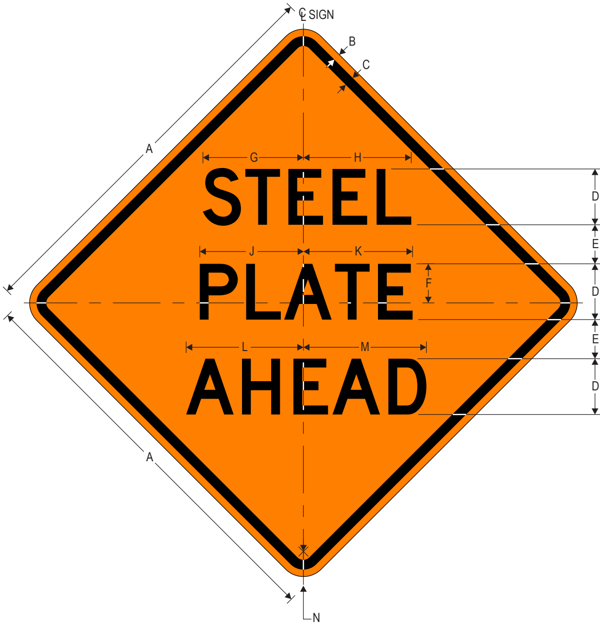
CW8-24 STEEL PLATE AHEAD
