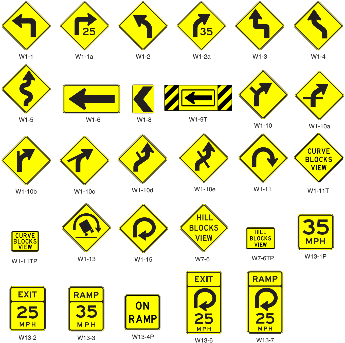
Figure 2C-1. Horizontal Alignment Signs and Plaques
