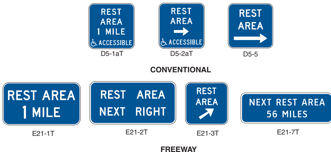
Figure 2I-5. Rest Area and Other Roadside Area Signs
