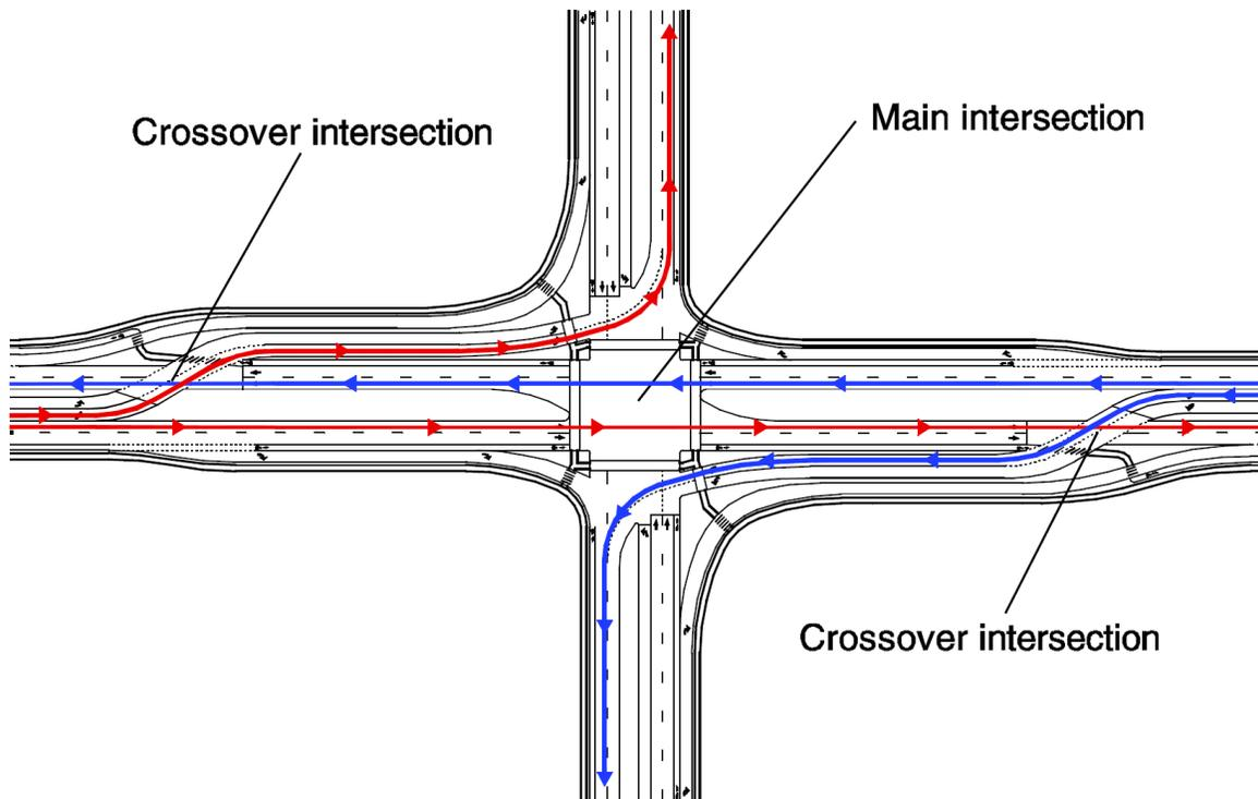
Figure 6-5 Example of a DLT intersection design sketch
