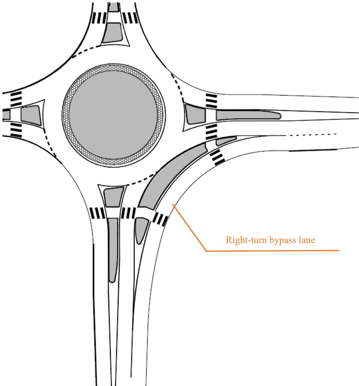
Figure 6-3 Example of right-turn bypass lane at a roundabout
