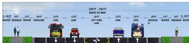
Proposed Roadway Typical Section
