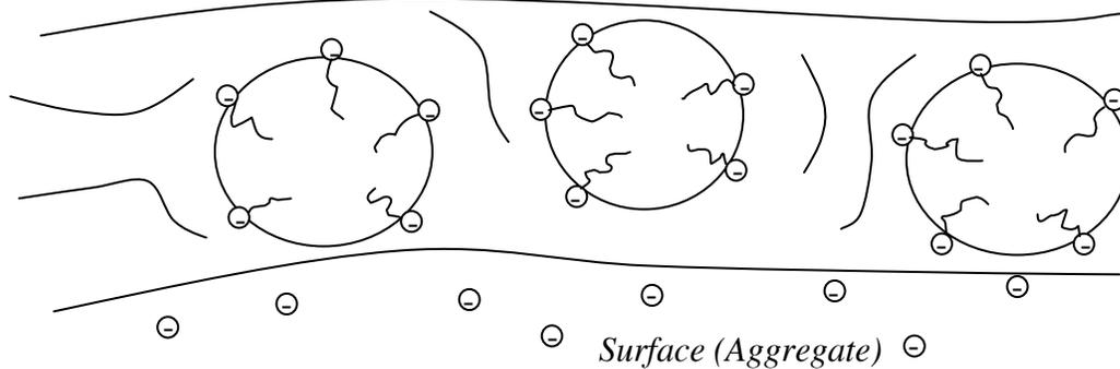
In an application of cationic emulsion, we are applying positively charged drops of asphalt to a negatively charged surface. The asphalt drops are immediately attracted to the surface and begin to break. The emulsion also loses water by evaporation. Thus the cationic emulsion has two breaking mechanisms at work and will break faster than a corresponding anionic emulsion. A depiction of the application is shown below.
